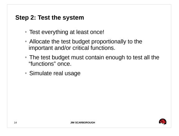
Slide 13: Now we need to plan testing. Test all your functions at least once, and allocate the test budget across the functions in proportion to their usage and severity of their failures. Ideal tests for this purpose simulate real usage.
